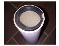
Figure 6b: Put Lens into tube followed with the final C-Ring on top.
