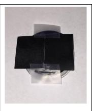
Figure 8a: Slit formed by 2 card rectangles
