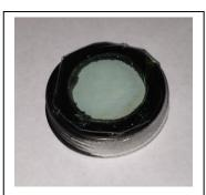
Figure 10: Hot Melt Glue the CD to the other end cap (inside).
