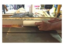
Figure 2a: Cut a slot in the 2" PVC pipe.
