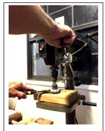
Figure 7: Drilling a 1" hole in the plastic endcaps.
